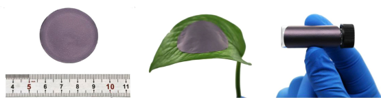
Fig. 16. The photograph of fabricated MXene paper with excellent flexibility. (Reprinted from [98] with permission: © 2019 Elsevier B.V.)
